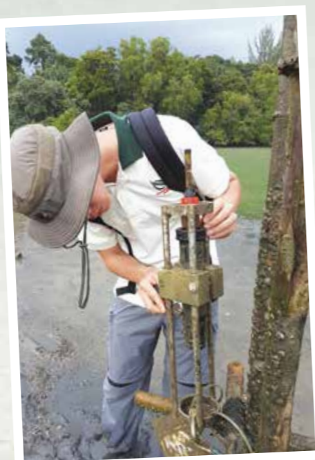
Collecting tidal data from the tide gauge Photo credit: Germaine Leng
